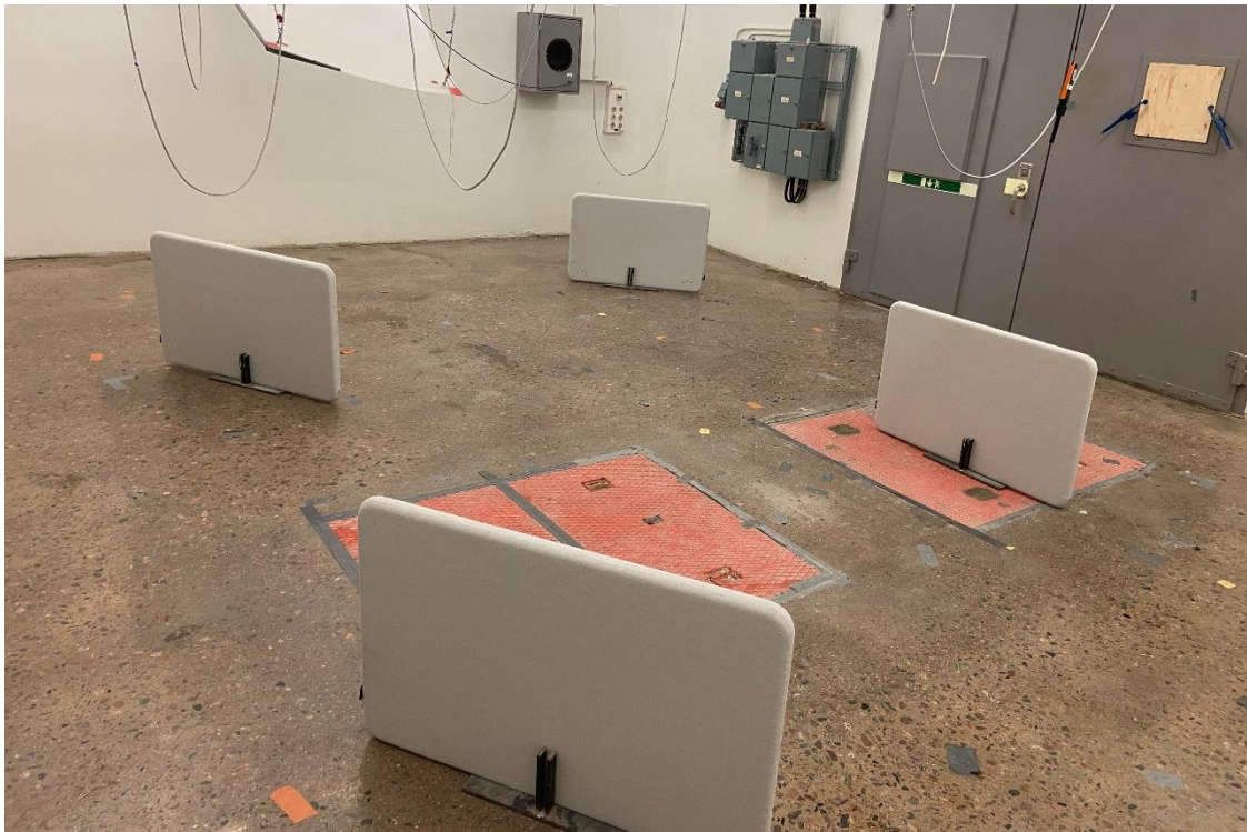
Figure 2. Acoustic front screen of type FONO for a 1000 mm long desk mounted in the reverberation chamber.
