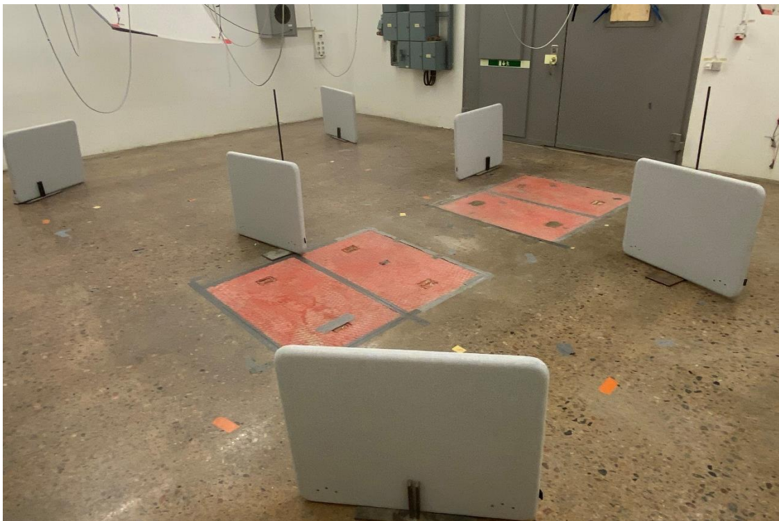
Figure 1. Quadrangle acoustic side screen of type FONO for an 800 mm deep desk mounted in the reverberation chamber.
