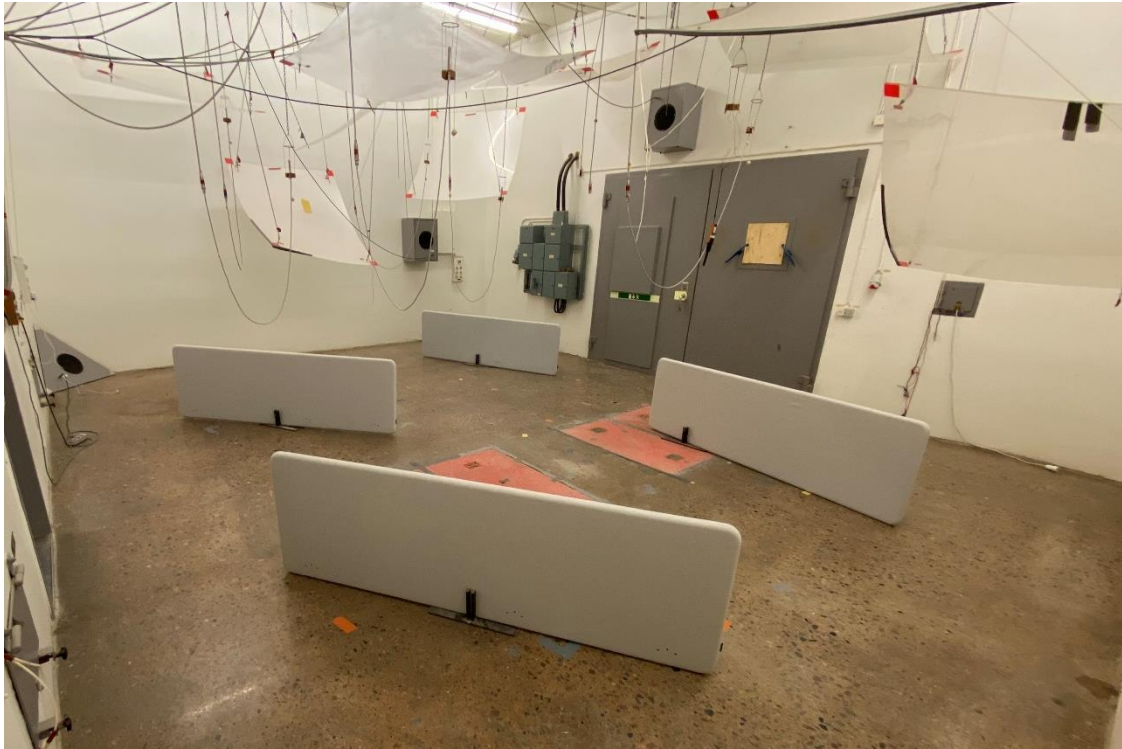
Figure 4. Acoustic front screen of type FONO for a 2000 mm long desk mounted in the reverberation chamber.
